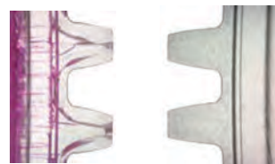
Stress cracked PC.
