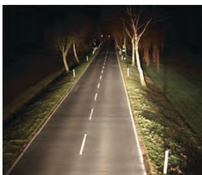
Typical light distribution and colour temperature of a light beam with standard halogen bulb.
